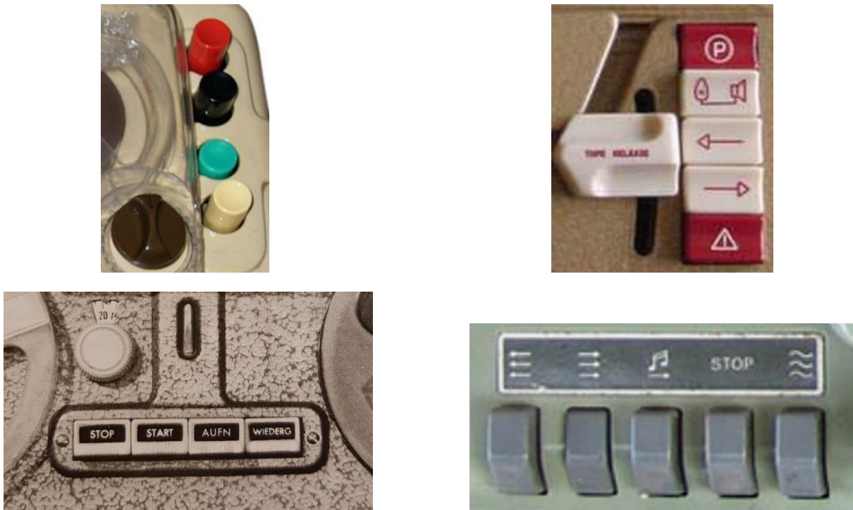
Figure 15: Operation buttons on, from left to right, first line: a Geloso G255 (1955), a Truvox R1 (1956). Second line: a Butoba TS6 (1957), a Revox F36 (1962). Without the manual, it was not evident to intuitively understand what the function of the buttons were.
